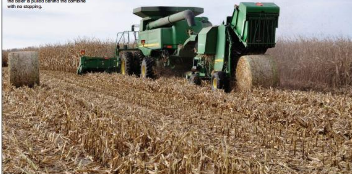
1-PASS BALING: The single-pass round baler system that Tim Couser has been testing makes stover bales on the go, as the baler is pulled behind the combine with no stopping.
