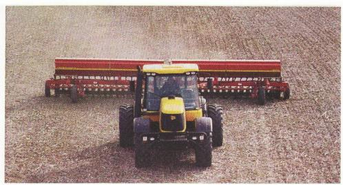
This is one of four new 30-foot grain drills used by FDC Enterprises to plant native warm-season grasses. Accurate planting depth is a must for good seed germination, and that means taking your time to avoid skips, bumps and bunches
