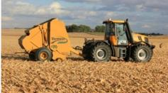
One version of Vermeer's 605 corn stover special lays bales out across the row. The goal of field testing is to identify the technology that speeds up and improves the efficiency of biomass collection. PHOTO: ANTARES GROUP
