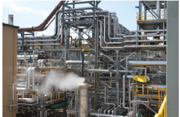
The Abengoa Bioenergy Biomass of Kansas uses an innovative process to convert a range of agricultural residues into sugars, which are then fermented, distilled, and dehydrated into denatured fuel ethanol for shipping distribution centers in the region. | Courtesy of Abengoa
