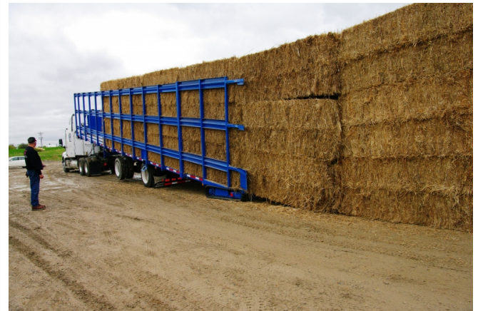
KELDERMAN SELF-LOADING TRAILER, OPEN SIDES Another version of the Kelderman Manufacturing Self-Loading Trailer, in action-picking up a stack of 36 corn stover bales in 5 minutes. Image: Photo courtesy of Dave Jordan, MacDon Industries Ltd
