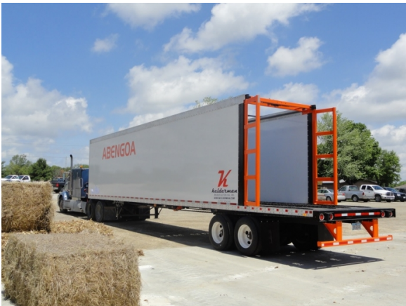
KELDERMAN SELF-LOADING TRAILER The Kelderman Manufacturing Self-Loading Trailer as adapted for Abengoa Bioenergy Biomass of Kansas biorefinery. Image: Photo courtesy of Kelderman Manufacturing
