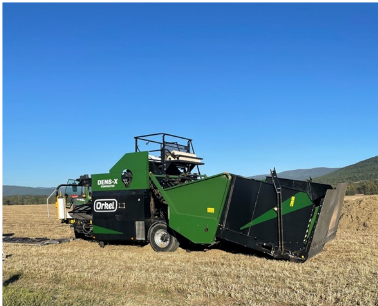
The Orkel Dens-X compactor, the highest capacity Orkel compactor.
