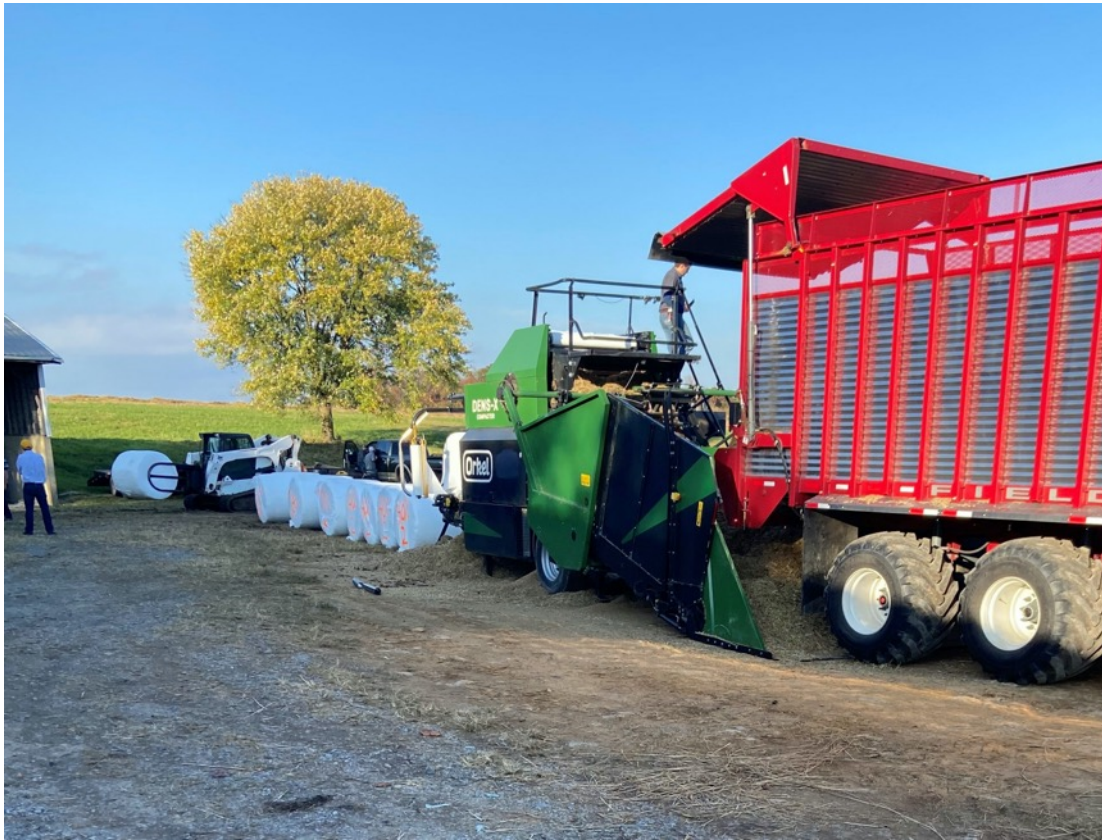
Baling miscanthus and switchgrass, two materials which the compactor model is highly compatible with.
